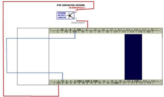
By connecting the COM connector with 24V, the X connectors will have the same 24V potential, this way the PNP versions of XC3 models(except XC3-14) can be used with NPN sensor as well:
